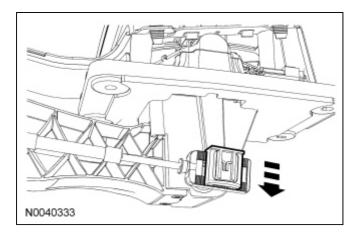
5. Verify the transmission selector lever cable is adjusted correctly. For additional information, refer to <a href="Selector Lever Cable Adjustment">Selector Lever Cable Adjustment</a> in this section.
