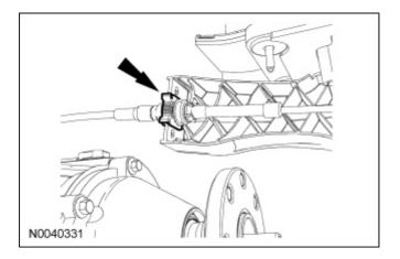
4. Remove the transmission selector lever cable from the transmission manual control lever.
