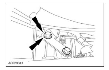
2. Install the transmission selector lever cable eyelet onto the transmission manual control lever.
