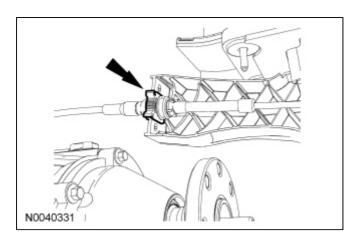
4. Install the transmission selector lever cable onto the selector lever and lock the selector lever cable adjustment lock.
