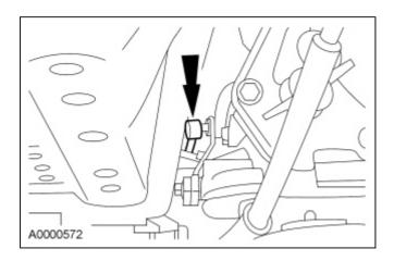
3. **NOTE:** It is necessary to install a new plastic transmission selector lever cable retaining clip prior to installation.
