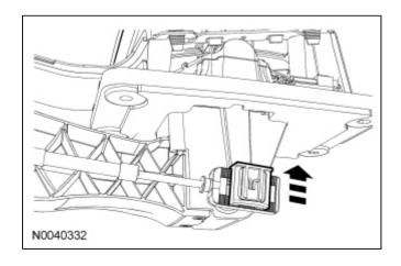
3. Remove the transmission selector lever cable from the transmission selector lever cable bracket and discard the transmission selector lever cable retaining clip.
