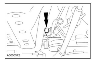
5. Remove the 2 transmission selector lever cable bracket bolts from the transmission and remove the bracket.
